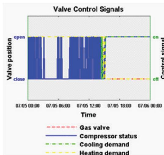
Figure 1: Temperatures and status points from the RTU with the cycling compressor on the day it was fixed. A little after midday, the compressor status stops cycling on and off, and the RTU supply temperature, which had been over 100 degrees, drops.
