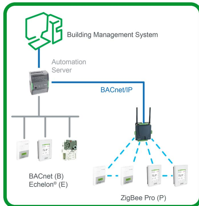
Figure 2: Simple diagram showing various wired and wireless systems in a single ecosystem
