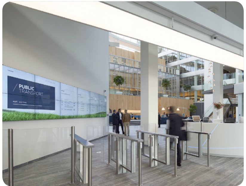
Real time energy consumption and efficiency data gathered from the SmartStruxure solution BMS are shared with building occupants and visitors via a dashboard located on a video screen located in The Edge lobby.
